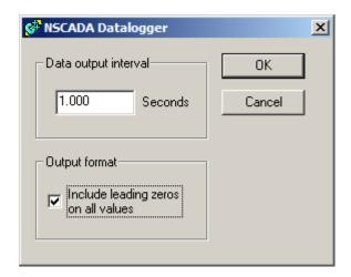
This dialog allows the Data output interval for the NORCOM Datalogger to be changed, from the default value of 1 second to the appropriate interval. It also allows the operator to include leading zeros on all output fields effectively making the telegram a fixed field fixed length telegram.
